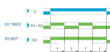
Function Di - Symmetrical flashing (ON Start)
